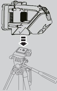
11. On the lower side of the lamp is a thread for mounting on all stands with 3/8"-16 UNC thread (Fig. 11).
