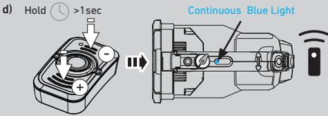
→ The main functions of the lamp can be controlled only via the remote control now.
